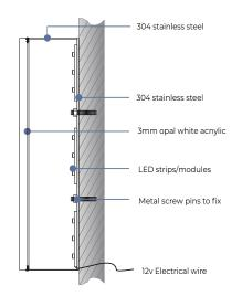
Face: 3mm / 4.5mm / 6mm Acrylic Body: 1mm fabricated 304 grade stainless steel
