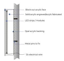
3mm / 5mm solid acrylic with block out colour Body: solid acrylic engraved/acrylic fabricated
