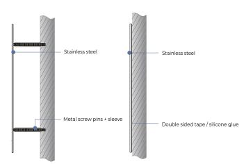
Stainless Steel - 1mm 3mm and 5mm (304/316 grade) with brushed/polished, painted, power coated, electroplated, aged / rusted, UV printed
