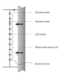
Material: 1.0mm 304 stainless steel fabrication (option for 316 stainless steel)
