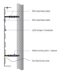
Face & Body: Fabricated 1mm 304 grade stainless steel (Option: 1mm / 2mm / 3mm 316 Marine Grade)
