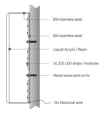
Face: 8mm-10mm Liquid Acrylic / Resin filled Body: 1mm 304 fabricated grade stainless steel
