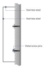
Face & Body: 1mm fabricated 304 grade stainless steel
